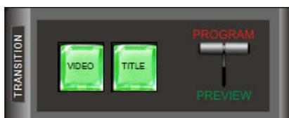
This panel has a PROGRAM/PREVIEW button that visually mimics the 'bar' control found on traditional hardware video mixers. The operation of this bar is described below associated with the operation of PREVIEW mode.
